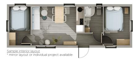
Meveline homes are fantastic alternatives to wooden and traditional homes. The homes are delivered pre-built and placed directly on the ground without a foundation. Because of the attachable wheels, they can be positioned anywhere. The home's mobility has a huge impact on the use as a temporary structure. Additionally, after placing the home at its permanent location you can mask the mobility function and aesthetically integrate it into the environment.
